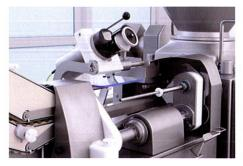
Ergonomic spooling position and optimised casing change function. DA 78-6 can optionally be attached.
