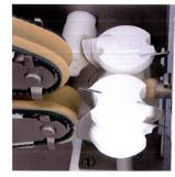
Newly developed voider permits up to 1,000 portions per minute in natural casing.
