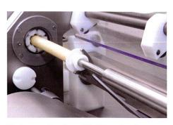
Casing pusher for artificial and collagen casings: Reliable linking and reduced non-productive times.
